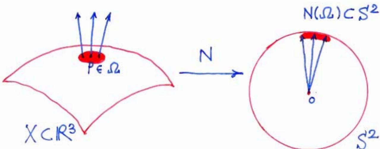
$$K := \lim_{\Omega \rightarrow P} \pm \frac{\text{Area}(N(\Omega))}{\text{Area}(\Omega)}$$
