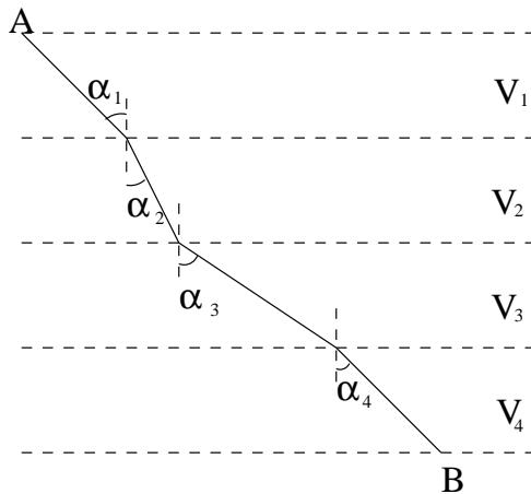
$$\therefore \frac{\sin \alpha_1}{V_1} = \frac{\sin \alpha_2}{V_2}$$
