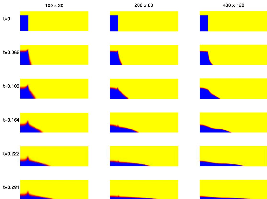
Figure 2: Pseudocolor plots of volume fraction for the broken dam problem. Results are shown at six different times obtained using the fluid-mixture algorithm with three different mesh points.
