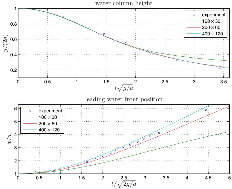
Figure 1: Comparison between numerical solutions and experimental results for the broken dam problem. On the top, results on the water column height are shown, and on the bottom, results on the leading water front position are shown. A mesh-refinement sequence  $2^i(100 \times 30)$  for  $i = 1, 2, 3$  are used for comparison. Here we have  $a = 0.06\text{m}$  and  $g = 9.81 \text{ m/s}^2$ .
