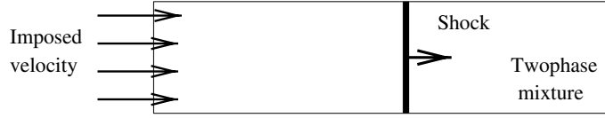
Fig. 8. Schematic representation of the two-phase impact problem.
