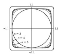
$$L_{2k} = 4 \int_0^1 \sqrt{1 + \left[ -x^{2k-1} (1 - x^{2k})^{1/(2k)-1} \right]^2} \, dx = 4 \int_0^1 \sqrt{1 + x^{2(2k-1)} (1 - x^{2k})^{1/k-2}} \, dx$$
